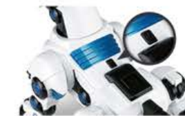
Reset Key: Dogo will stand up once press reset key
